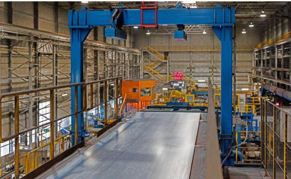
The entry gauge is arranged between the bridle rolls and the entry of the pickling section (Picture: Salzgitter Flachstahl)
