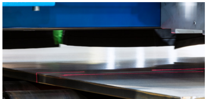
The measuring system projects laser lines onto the plate surface
