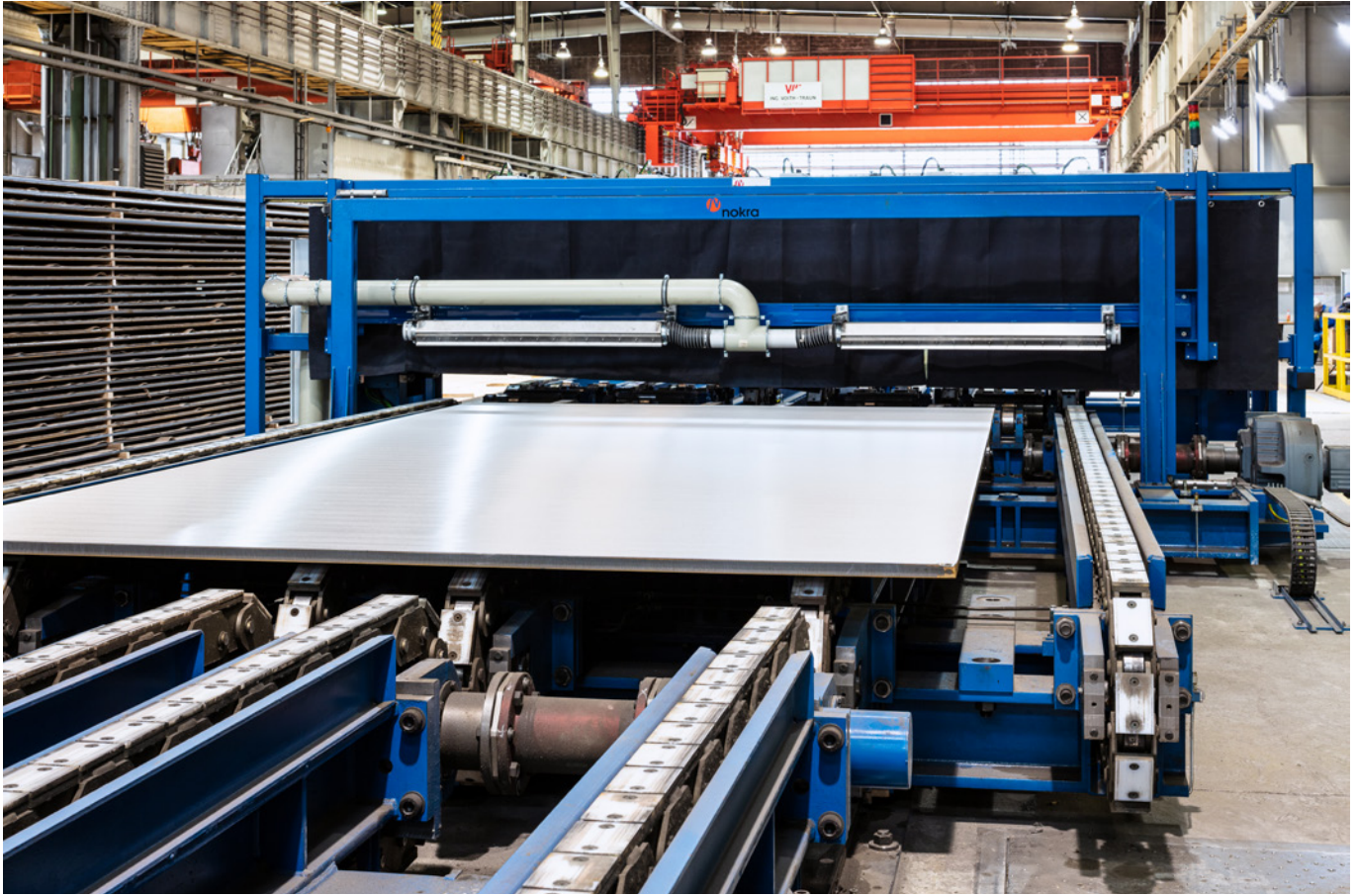
A roll-bonded plate entering the new measuring system
