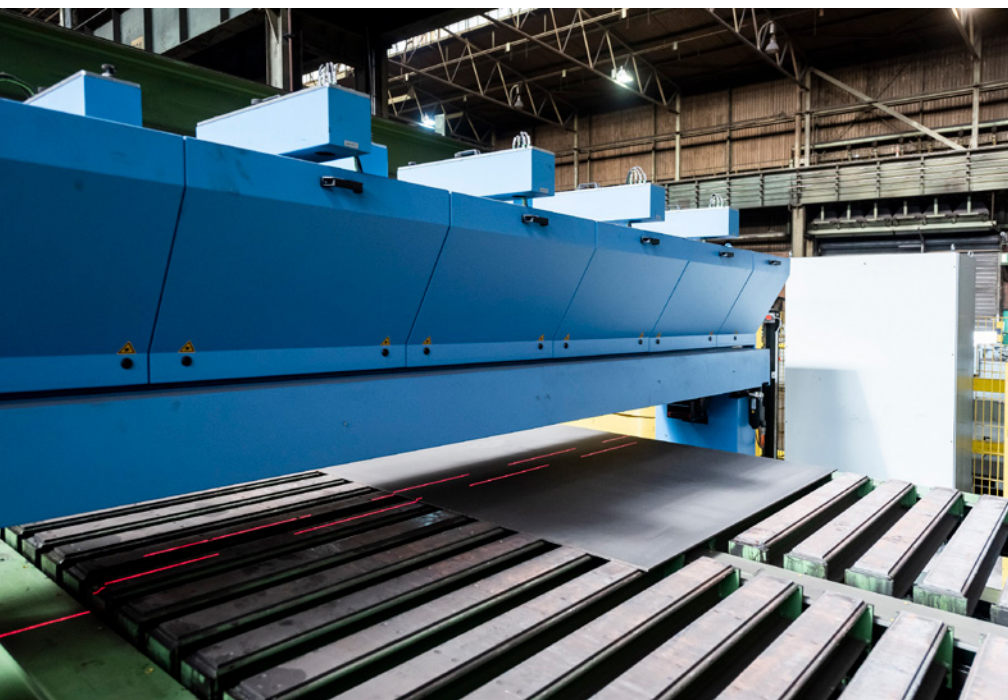
The flatness gauge is arranged at the end of the finishing line, behind the descaling and colour spraying line (Picture: thyssenkrupp Steel Europe)
