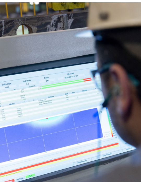
The plate topography is rendered in a false-colour 3D view or a plain view from above (Picture: thyssenkrupp Steel Europe)
