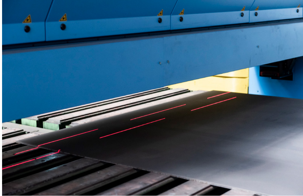
The laser lines projected by the individual sensors are offset to avoid any misinterpretation of camera signals (Picture: thyssenkrupp Steel Europe)
