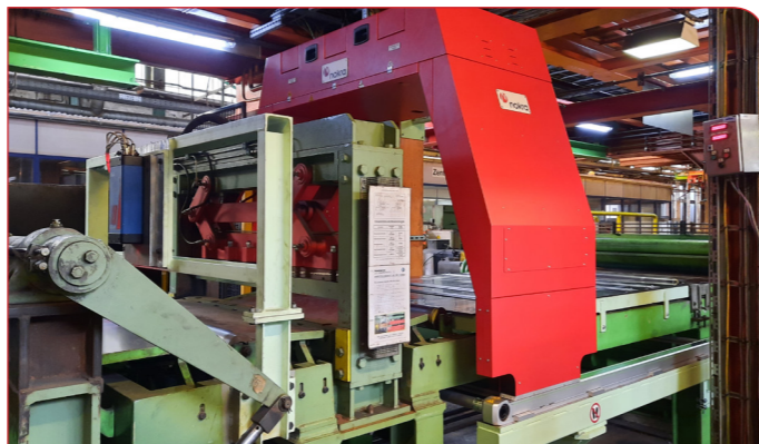
Figure 2: The measuring portal in the parked position ahead of a cut-to-length shear
