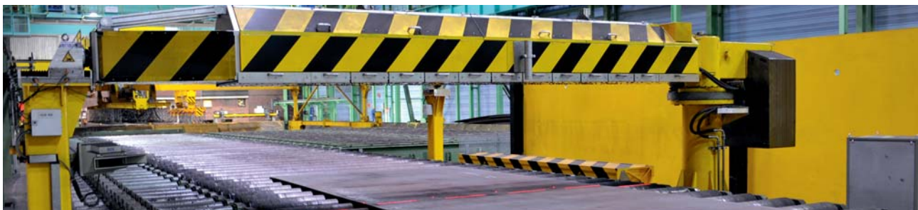
Fig 4: nokra flatness measurement system alpha.fi at a plate mill
