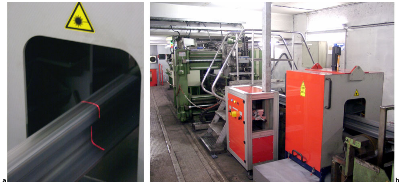
10 a profile measurement at rails running through measuring unit and b view of profile measurement system in rail inspection centre (source: TSTG Schienen Technik)
