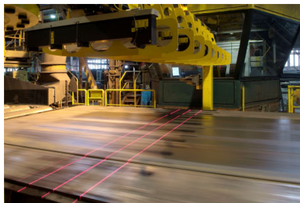
2 Flatness measurement with lasers downstream of leveller in heavy plate rolling mill, measuring field with three laser lines (source: ThyssenKrupp Steel)
