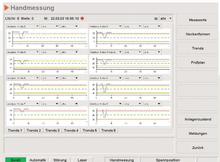
Trend display allows the timely correction of upstream processes
