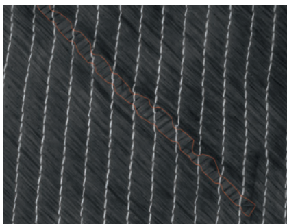
Fig. 3. The system recognizes gaps in the structure
