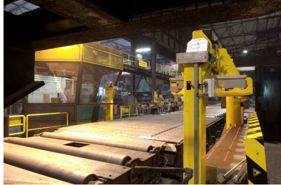
(Pic.3 Measurement gantry in alignment position)
